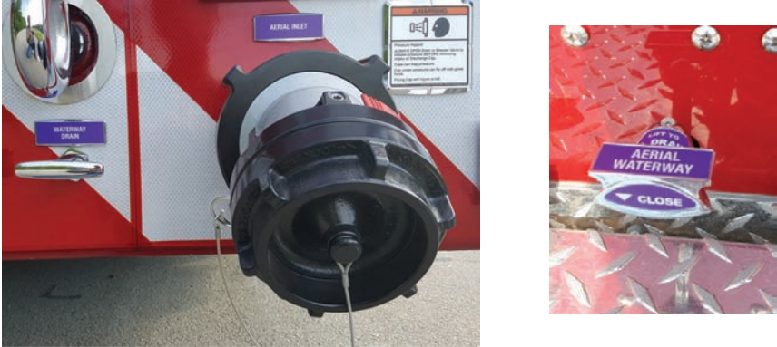
Figure 3-24. Waterway Drain and Aerial Inlet
