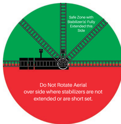
Figure 4-5. Short Set Rotation Interlock Stop Points
