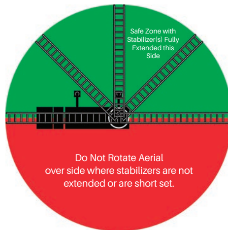
Figure 2-2. Short Set Rotation Interlock Stop Points
