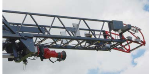
Figure 4-14. Monitor at the end of next lower ladder section
