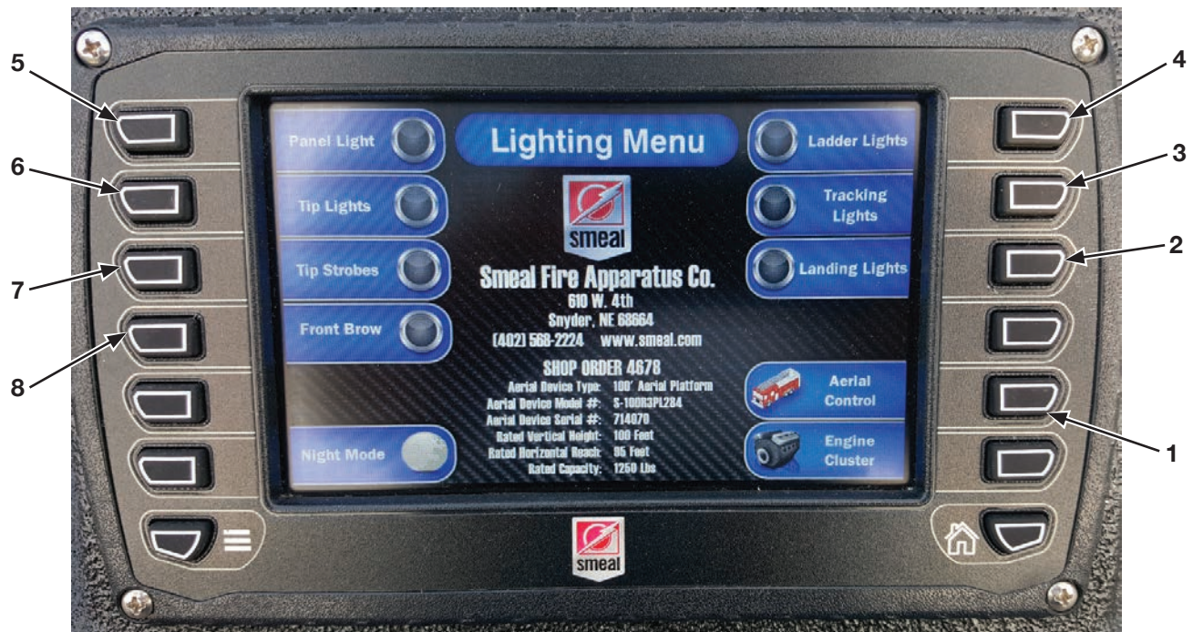
Figure 3-13. AL-11 Lighting Control Screen
