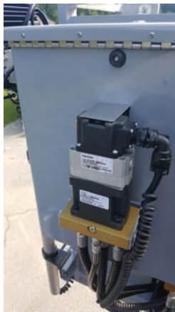
Figure 4-21. Manual Emergency Platform Bucket Leveling - Servo-Valve Control Under Cover
