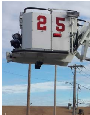
Figure 4-6. Maintain Sufficient Clearance
