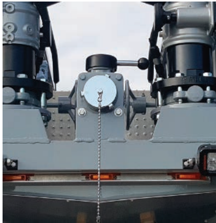
Figure 4-13. Aerial Standpipe Connections 2-1/2 in. and 1-1/2 in.
