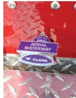
Figure 3-23. Waterway Drain and Aerial Inlet
