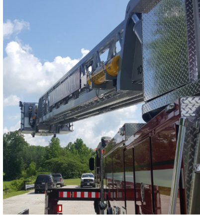
Figure 3-18. Ladder Movement Stops Prior to Contacting Body of Apparatus
