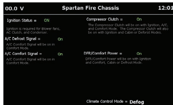
Figure 3-34. HVAC Diagnostics for Dual Overhead System
