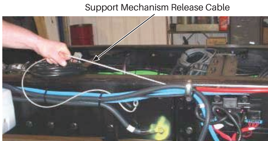
Figure 3-2. Lowering Cab - Safety Support Mechanism Release Cable
