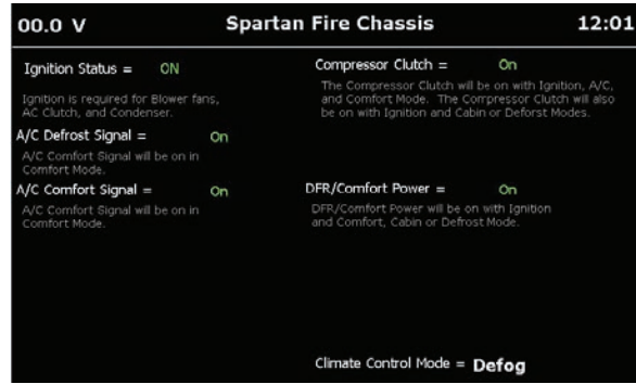
Figure 3-35. HVAC Diagnostics for Single Overhead System
