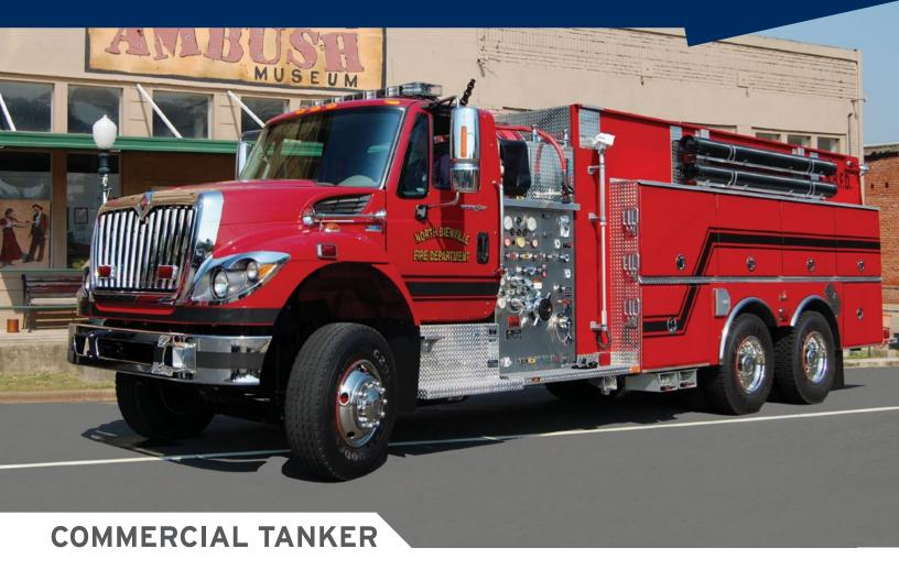
Available in 4-door or 2-door, Commercial Tankers from Ferrara are built fire service tough. Using heavy duty construction on every vehicle, Ferrara Commercial Tankers are extremely durable. Available with tank sizes up to 4000 gallons and in a traditional pumper-tanker body, wetside or elliptical tanker design, these trucks will provide the additional performance flexibility your fire department needs when keeping your community protected.
