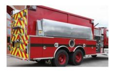
Hydraulic portable tank rack
