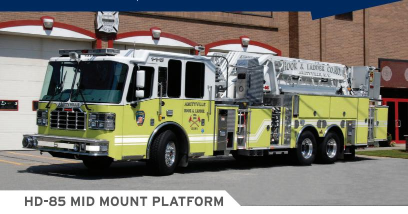
Designed for traditional truck company operations, the Ferrara HD-85 Mid Mount Platform boasts over 300 cubic feet of usable compartment space and the ability to carry up to 200' of ground ladders. Couple this with the ability to reach a 5th floor building and overcome a set-back of over 70 feet, and you'll want to learn more about the HD-85.
