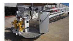
Ferrara's optional rope rescue/lifting arm also doubles as a temporary stokes mount
