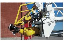
Quickly put out a fire in an attic or upper void area with our optional 165 vertical travel monitor
