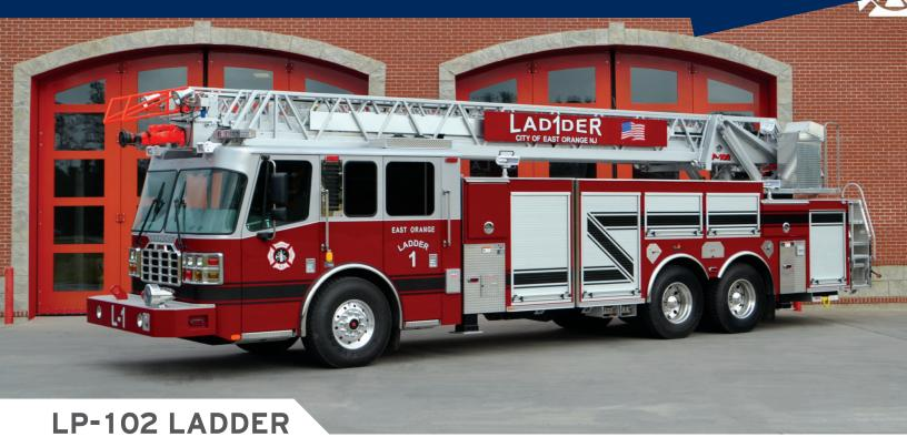
The LP-102 is the perfect solution when you are faced with a smaller fire station that not only has small door openings, but also limited in the length of vehicle that can be kept. The LP-102 can be built as low as 10' 10" with a pre-piped waterway and 10' 4" without waterway. If needed, the truck can also come in under 40' overall length.
