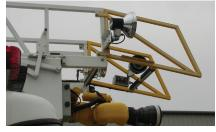
Standard 11° angled, bolt-on egress section for easy transition to a window or roof
