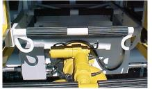
Standard pair of load lifting eyes at the ladder tip are rated at 500lbs as a pair for added rescue capability
