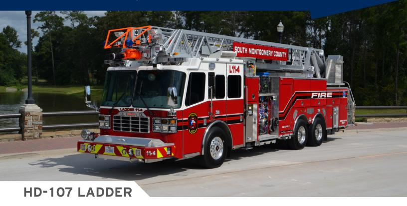
You want Heavy Duty? Then get Heavy Duty! Nothing says that like the Ferrara HD-107. Built with an impressive 750 pound tip load while flowing 1500 gpm in any ladder configuration, the HD-107 can be designed as a traditional truck or a quint with up to a 650 gallon tank.
