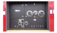
F-Shield, anodized aluminum or stainless steel pump panel treatments
