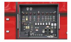
Open or enclosed rear pump control panel
