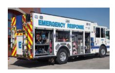
Industrial MVP Rescue Pumper 2000 gpm with Williams WATP 1500 Foam System
