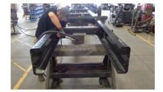
Double and triple channel, heat treated frame rails
