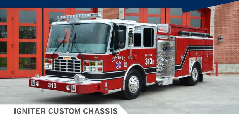
Descending from the Inferno, the Igniter offers the same heavy duty construction and performance that fire departments have relied on for years. This chassis features medium block engines and is available in two different widths with multiple cab, seat and equipment configurations. The Igniter is built to endure the rugged demands of high frequency runs by any metropolitan fire department.
