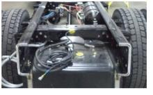
Double channel, heat treated frame rails
