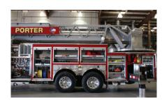
Carry more gear with rescue style compartments with openings on the driver side is 24" deep x full height
