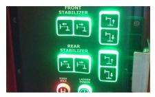
Our outrigger controls are waterproof, rubberized push buttons, which are function illuminated for fast setup
