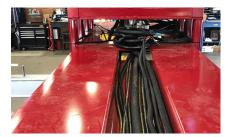
The top of the torque box has a recessed channel to accommodate wiring and hydraulic lines
