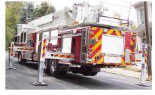
Optional increased stroke outriggers provide additional leveling capabilities up to an 11° grade
