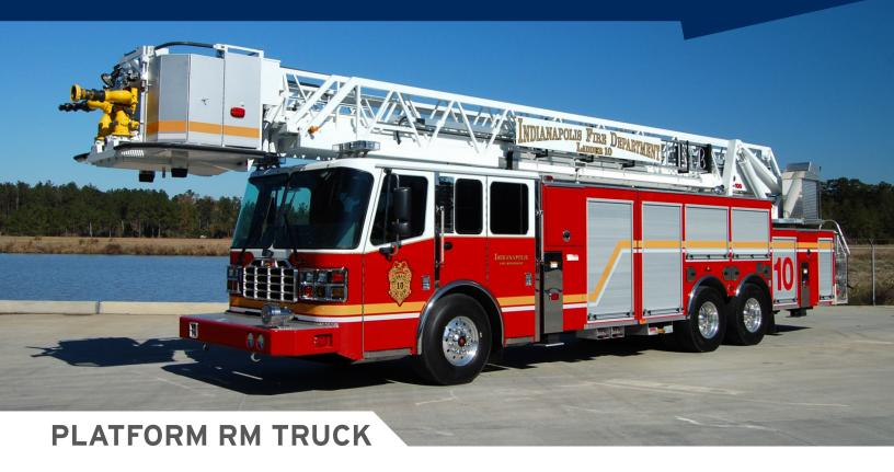
Safety. Heavy Duty Construction. Performance. These are all qualities you look for in an aerial platform. The Ferrara Rear Mount Platform gives you those and more. It also boasts Ferrara's legendary heavy duty construction with 3/16" thick aluminum cab and body plus a 100,000 psi steel aerial. For safety, the aerial has a full complement of safety interlocks, the cab and body have been load tested to 66,000 pounds in excess of NFPA 1901 requirements.
